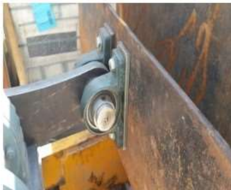
Plate 3: CAMA and pin connected during manufacturing of shaking box.
