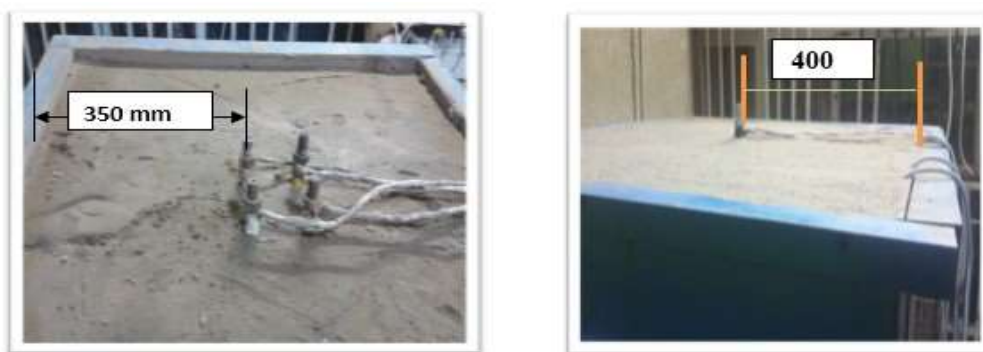
Plate 1: Clear distance between the pile and tank side.
