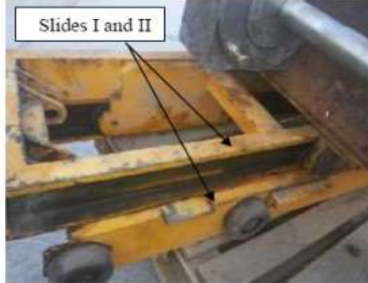
Plate 2: Slides and base bracket system during manufacturing of shake box.
