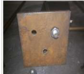
Plate 6: Steel plate used as pile cap and payloads.
